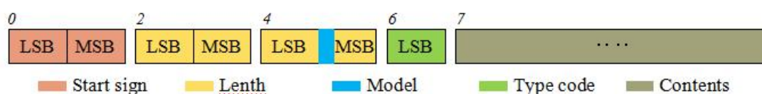
FIG 3 YDLIDAR G4 SYSTEM MESSAGE DATA PROTOCOL
